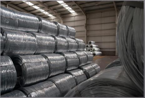
Wire is packed in coils of 500 – 800kgs
